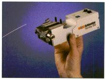
ing and dwell time system and rate of controlled stripping system. Special grippers are available for use with jacketed cables; an adapter is available to accept fusion splicer fiber holders.
