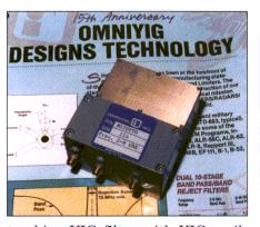
tracking YIG filter with YIG oscillator. The filter covers a frequency range of 2.0 to 8.0 GHz, with the oscillator offsetting by 160 MHz above the filter. The RF power output is +13 dBm minimum, with FM noise at -120 dBc at 100 kHz away. The unit is built to Mil-E-5400 specification andscan be integrated with an analog driver or 12-bit digital driver to tune the full frequency range. Operating temperature range is -54 to +85 degrees Celsuis. **Omniyig, Inc.**
