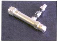
features high isolation and a 100-watt power capability over the cellular/GSM, PCS/DCS and UMTS frequency bands at 800 to 2200 MHz. A special feature of this model is the wideband isolation of the RF path from spurious DC power line interference. Model HW-11N is specified to reject all spurious signals from 500 to 2500 MHz by at least 50 dB.
