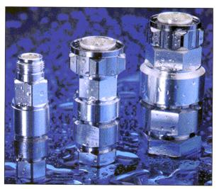
designed for quick and reliable in-field assembly in the radio base station environment. These connectors are available in N and 7/16 interfaces designed for several sizes of corrugated copper cables, including 1/2, 3/4, 7/8, 1 1/2 and 1 5/8 inch. All QUICK-FIT connectors are rated IP 68 using a three-stage sealing concept that waterproofs the jacket, outer conductor and connector interface.
